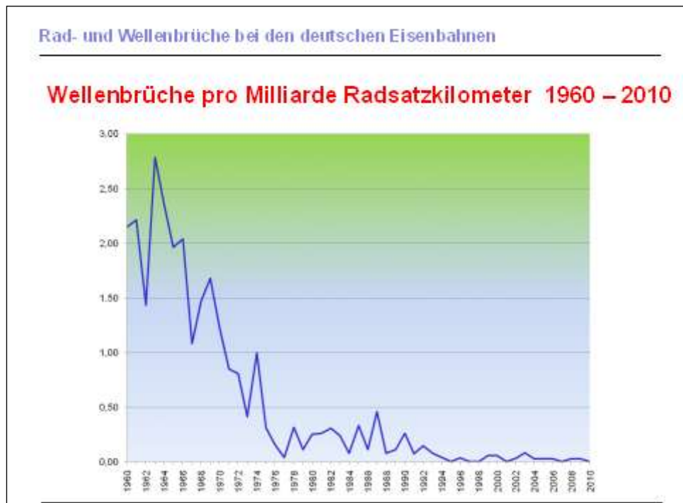
Figure 4: number of axle breaks per billion wheelset kilometers between 1960 - 2010
